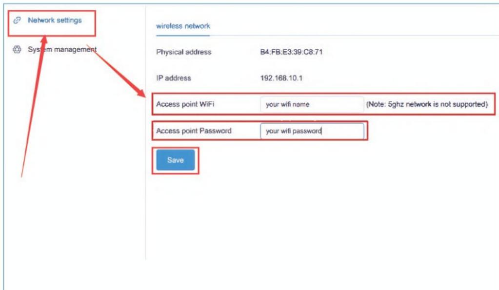
The screenshot shows a web interface for network configuration. On the left is a sidebar with two items: 'Network settings' (with a link icon) and 'System management' (with a gear icon). Both are enclosed in red boxes. Two red arrows originate from the 'Network settings' box: one points to the 'Network settings' text, and the other points to the 'Access point WiFi' input field. The main content area is titled 'wireless network' and contains the following fields:
